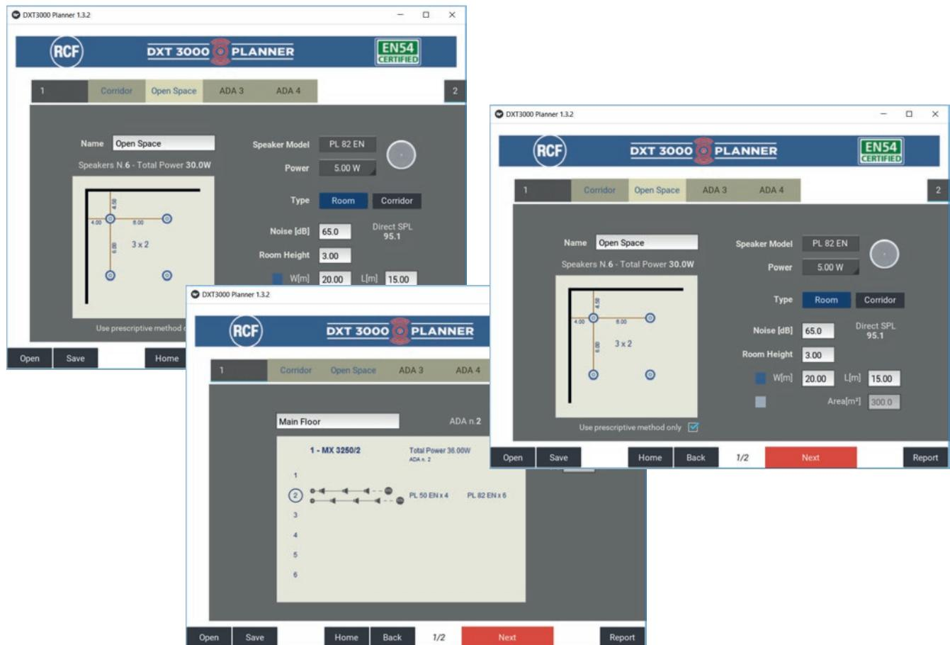
6. The result of all the above-mentioned deployment produces a PDF document containing the list of the EN 54 certified products necessary for the project. For each ADA a lists of the speakers with their possible theoretical distribution pattern in the environment is provided, in addition to the power tapping to set the speakers themselves.
