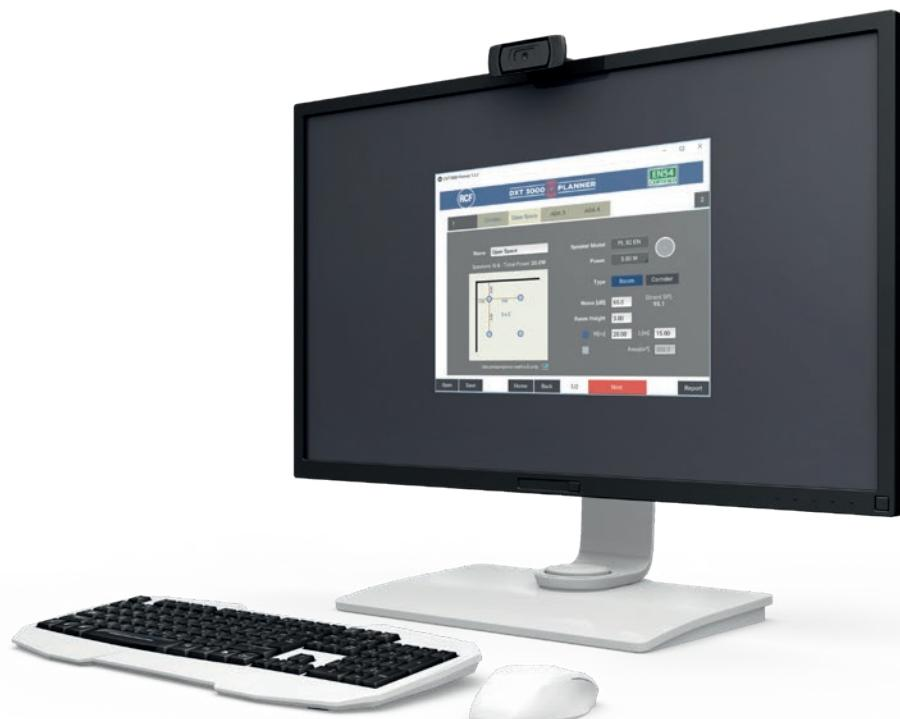
The Windows PC DXT 3000 Planner software allows configuring small and medium VOICE-ALARM systems in accordance to the regulations (prescriptive method), using EN 54-24 loudspeakers and EN 54-16 management electronics of the RCF DXT 3000 Series (250W and 500W models; 2, 4 and 6 zones, in stand-alone or networked configuration) and related accessories.
