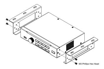
Position the unit to a spot under the desk where you can easily access the front-panel pushbuttons, and then secure the racks to the desk with selfprepared screws.
